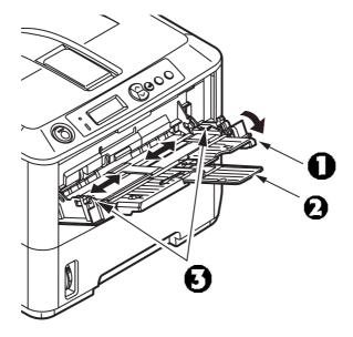
2. Insert a sheet of Letter/A4 plain paper between the paper guides and push the colored set button to engage the tray.
